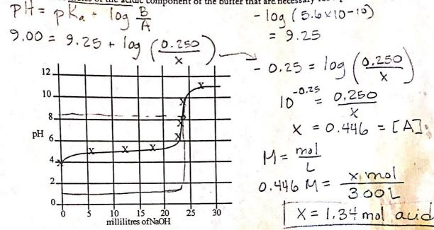
A 30.00 milliliter sample of a weak monoprotic acid was titrated with a standardized solution of NaOH. A pH meter was used to measure the pH after each increment of NaOH was added, and the curve above was constructed.
